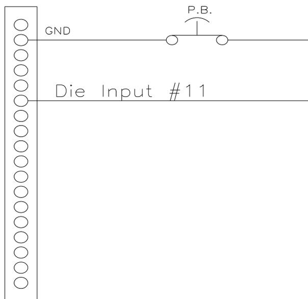
**Figure 7-4** Connecting Die Input #11 to Remote Circuitry
