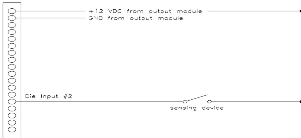
**Figure 2-6** Voltage Sensing Device
