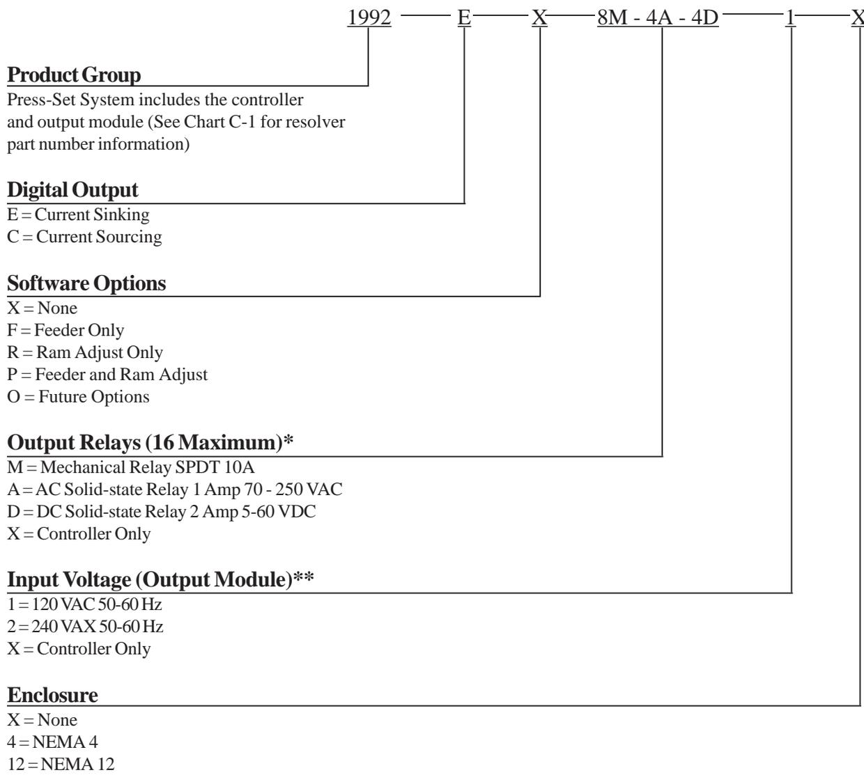
\* Any combination of mechanical, AC solid-state, and /or DC solid-state output relays can be selected, up to a total of 16.
