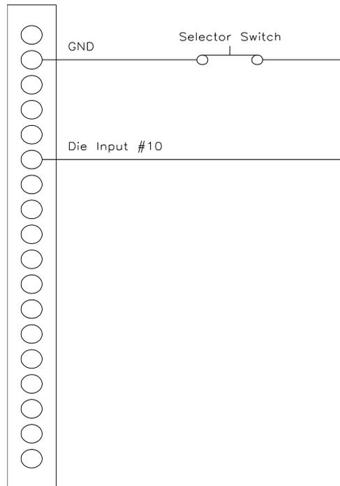
**Figure 6-5** Connecting Input #10 to Push Button
