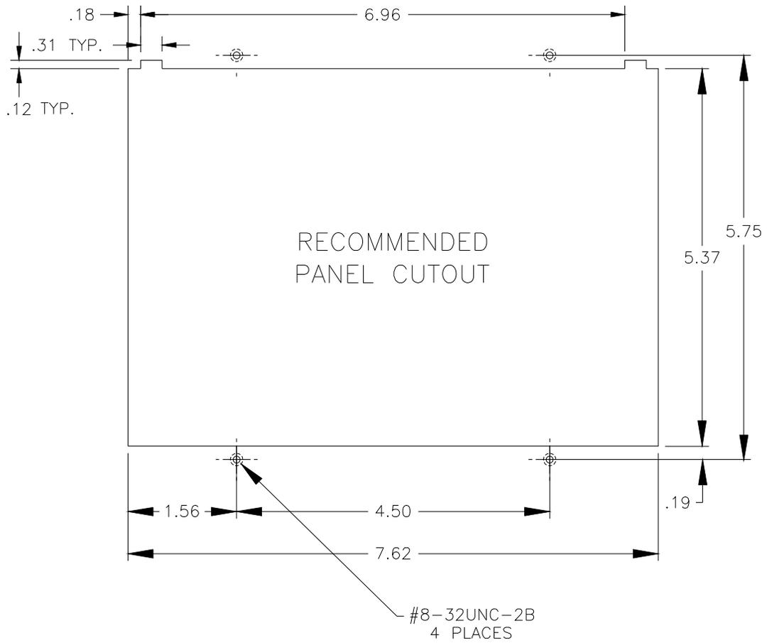
**Figure 2-1** Controller's Cutout Dimensions
