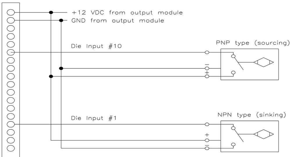
**Figure 2-7** Open Collector Devices, Photo Switches, Proximity Switches, ETC.
