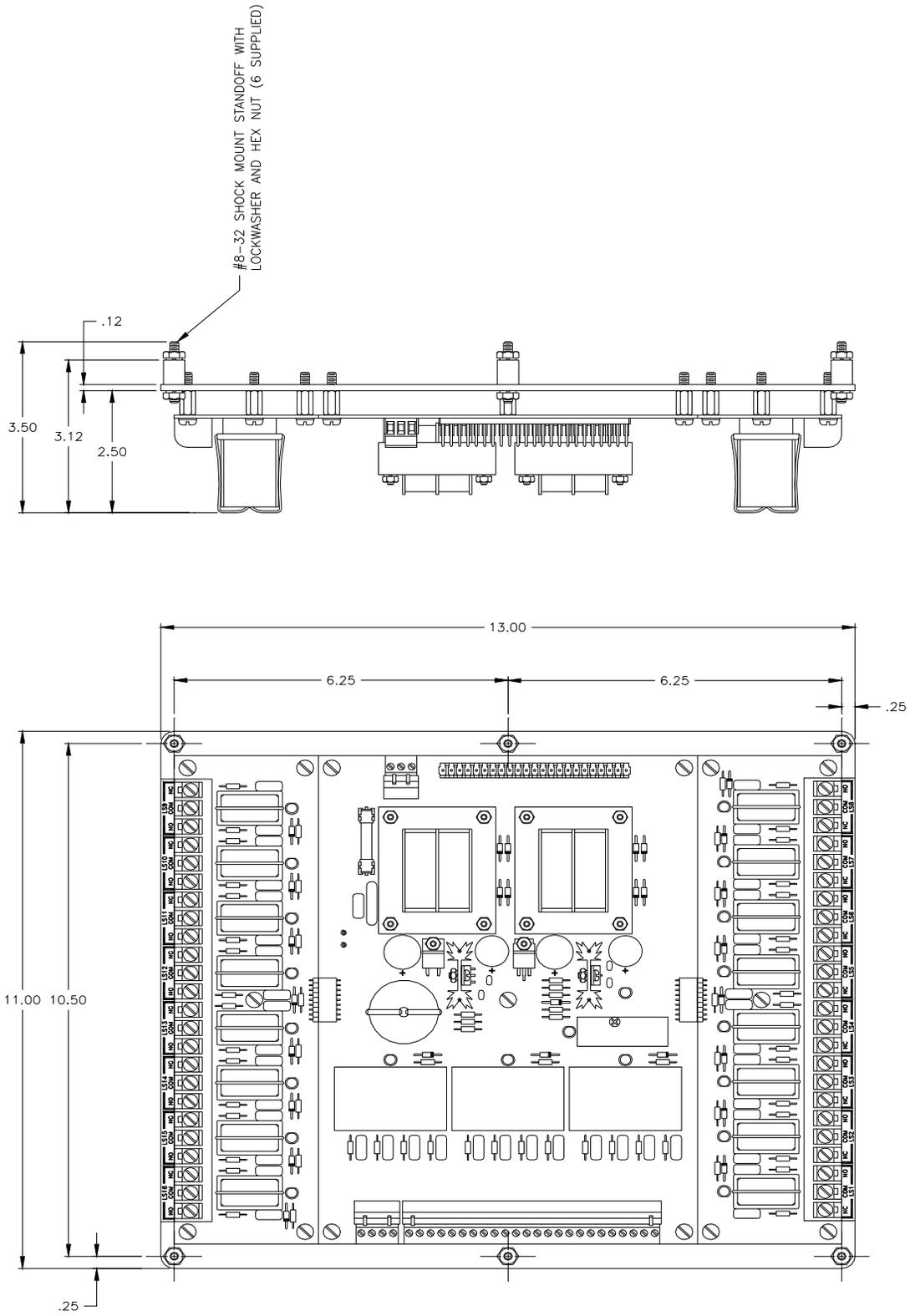
**Figure 2-3** Output Module's Dimensions
